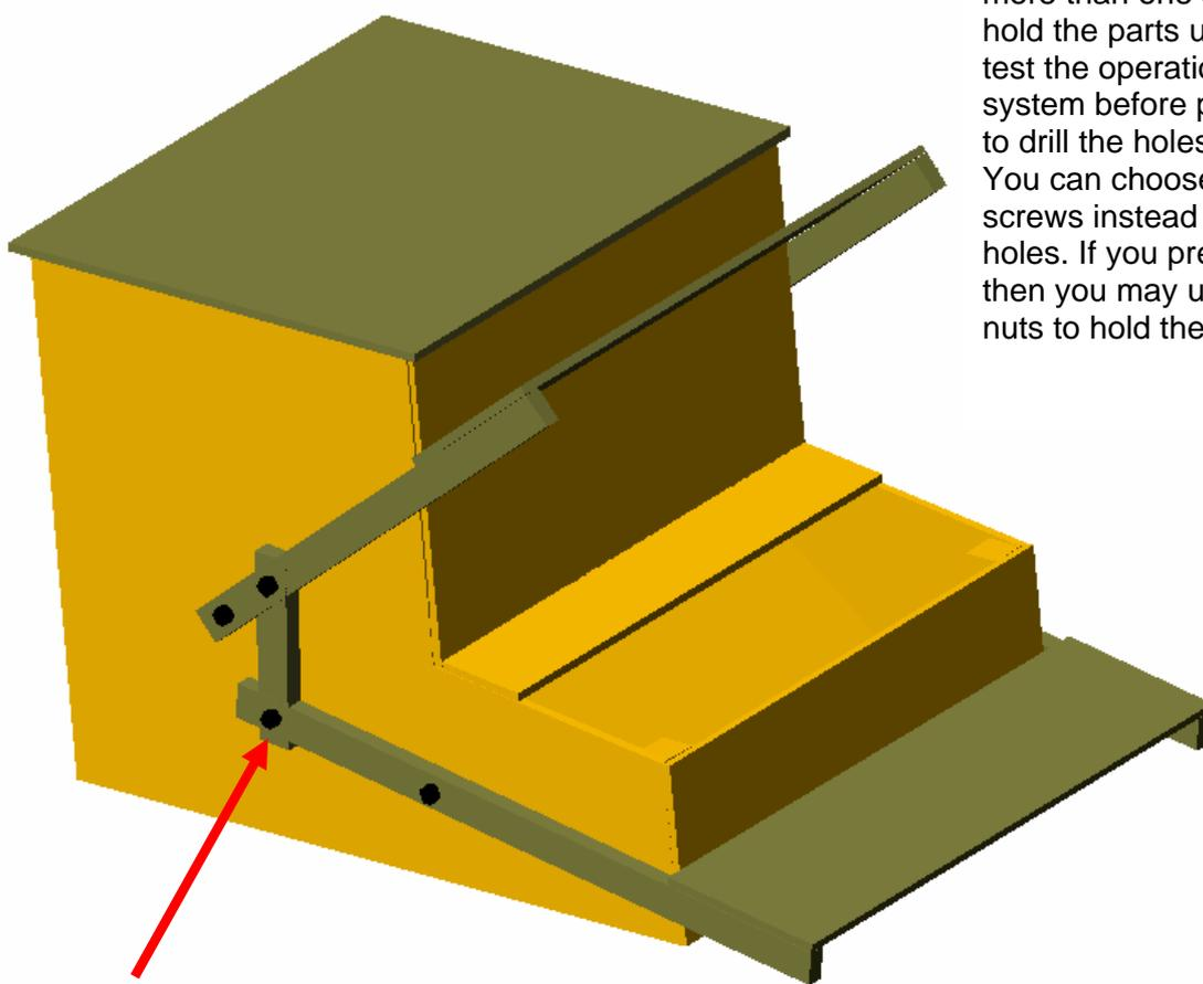
You can make holes for more than one setting, or hold the parts using nails to test the operation of the system before proceeding to drill the holes. You can choose to use screws instead of drilling holes. If you prefer drilling, then you may use bolts and nuts to hold the parts.
