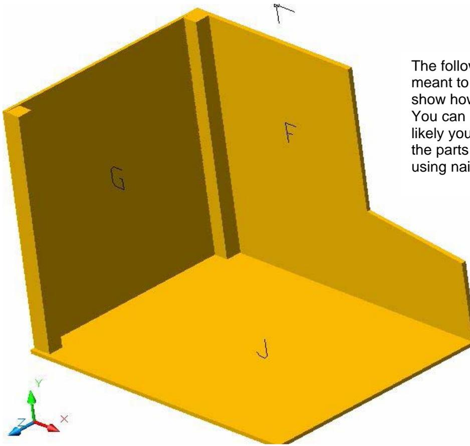
The following pictures are not meant to be steps but intend to show how all parts fit together. You can use wood glue but most likely you will need nails to hold the parts together. I suggest using nails of 3/4 or 5/8 inch
