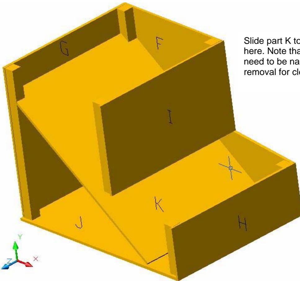
Slide part K to rest of G as shown here. Note that this part does not need to be nailed. This will allow removal for cleaning if needed.
