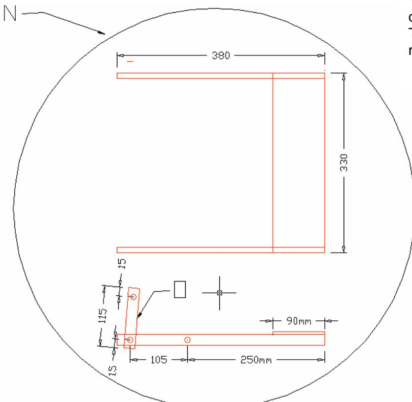
You may like to wait until the end to drill the holes on the moving parts. These distances should work but may need some adjustments.
