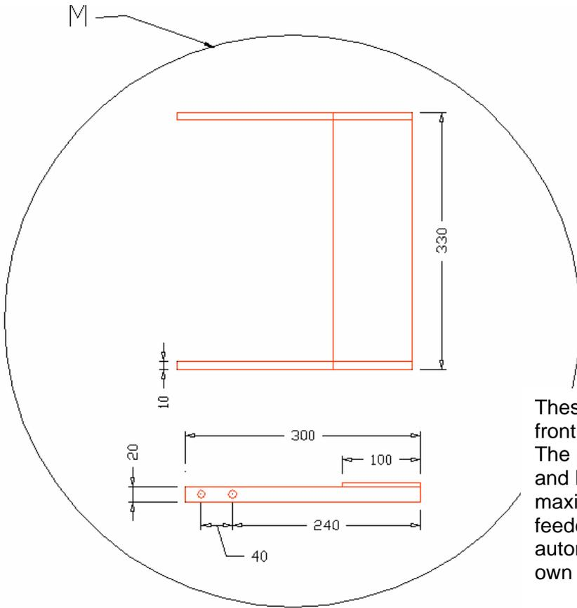
These diagrams show the top and front views of moving parts M and N. The position of holes on parts F, M and N have been selected to maximise the bird weight (to open the feeder cover) and to allow the automatic closing of the cover by its own weight.
